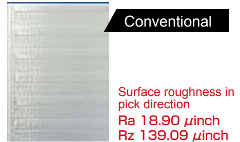
Cloudy and uneven milled surface with conventional tools
