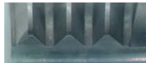
Epoch Thread Mill after threading 300 holes.
