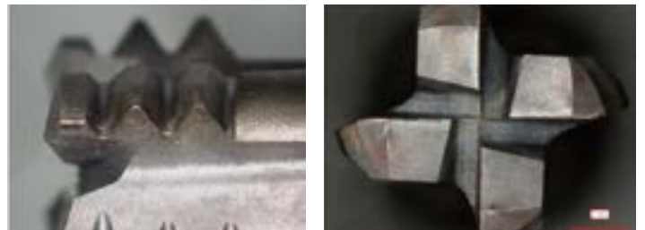
Epoch D Thread Mill after threading 50 holes.
