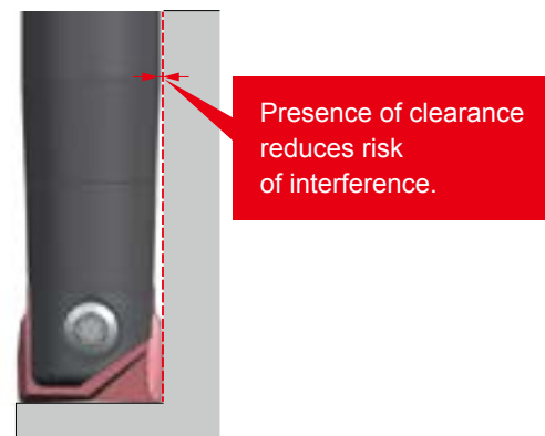
When insert with diameter +1mm larger than shank diameter is mounted.
