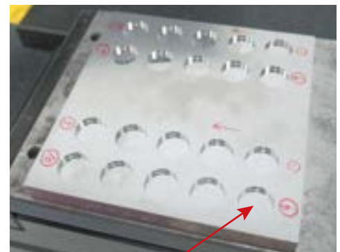
Machining shape \phi .347 \text{ inch} \times \text{Depth } .059 \text{ inch}
