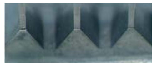
Epoch Thread Mill after threading 300 holes.
