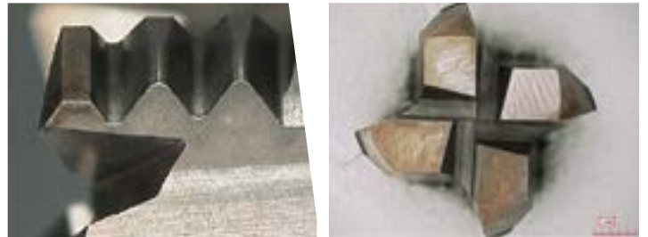
Epoch D Thread Mill after threading 64 holes.
