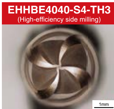
Flank wear : 0.015mm
