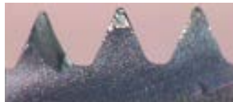
Conventional after threading 10 holes.
