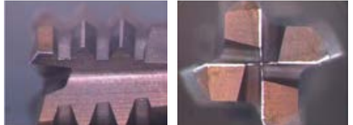
Epoch D Thread Mill after threading 600 holes.
